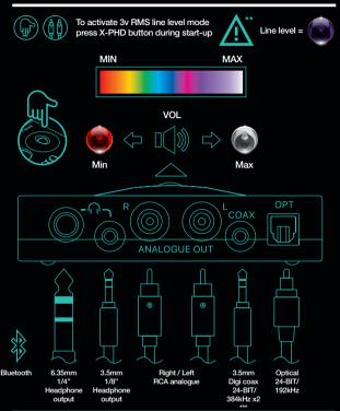
Coax 1 configuration = Tip and sleeve, Coax 2 configuration = Ring and sleeve. The 3.5mm digital coaxial lack input supports 'dual data mode', where 768kHz files can be input as two separate 384kHz data streams, should devices support this capability.
