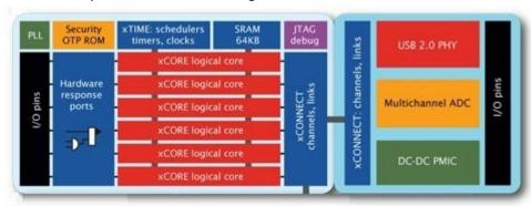
The IDAC 2 implements Version 4 AMR XMOS Platform and uses the latest generation 8-Core 500MIPS XMOS1 transputer derived main processor. These processors are quite unique in their architecture and are based on a technology that once was considered to have revolutionized computing, the INMOS Transputer: which allows extremely high sample rates, supporting 384kHz/32Bit PCM and 11.2MHz single bit (DSD).
