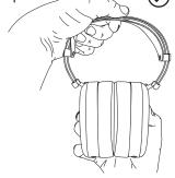
Place foam block between ear pads. Hold the headphone by the headband with one hand, grip both cups with the other hand as shown. Gently squeeze the cupts to keep them together while folding.
