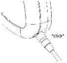
All Dan Clark Audio planar-magnetic products use Hirose-style connectors. To attach your cable hold the male connector by the boot and rotate it into the female receptacle on the headphone until you feel it click into place. To release the cable, pull down on the top of the connector's metal jacket.
