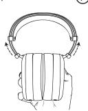
Move the sliders up until the leather is against the titanium headband.
