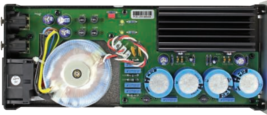
The linear power supply has a compact toroidal mains transformer (left), a bank of four cylindrical smoothing capacitors and heat sink (top right) for the regulator.
