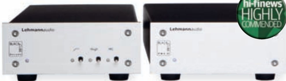
ABOVE: Here the neat front panel switches select MM or MC sensitivity, add 10dB extra gain, or engage a subsonic filter
