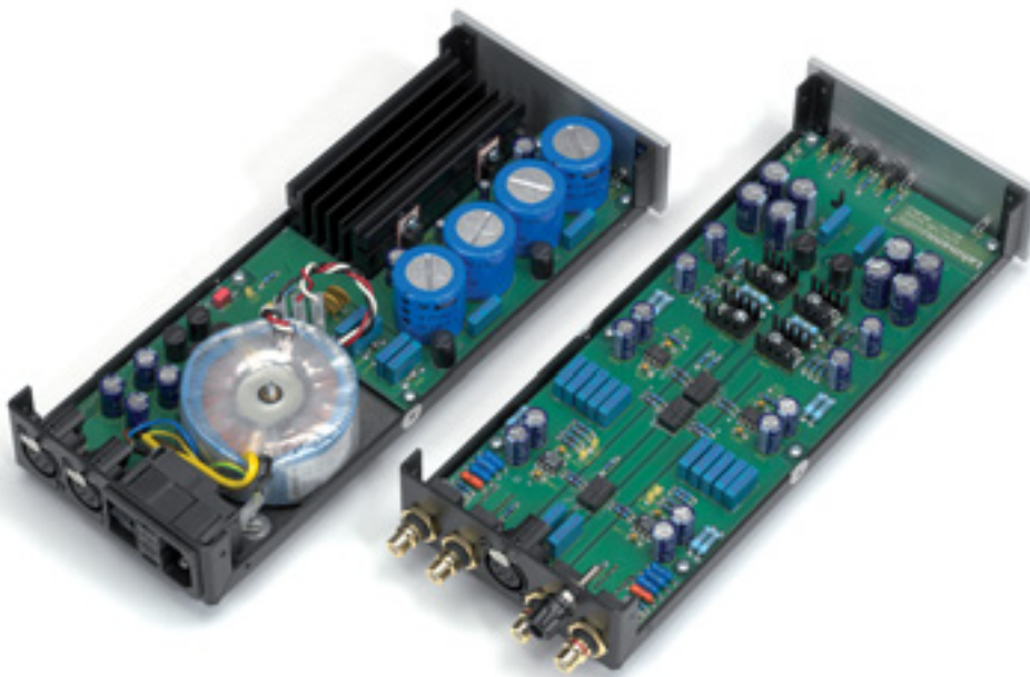
Professional craftsmanship, high-quality components, a sophisticated power supply, easy capacitance and resistance matching via DIP switches
