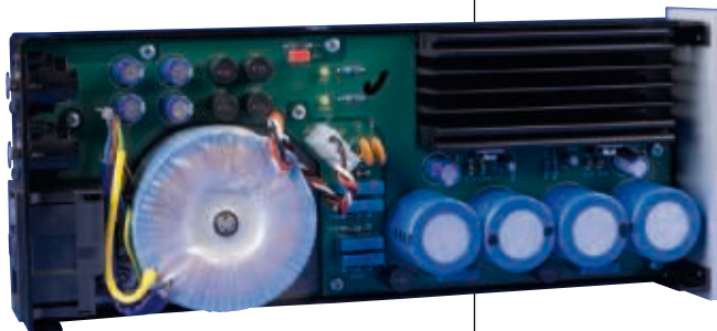
For a phono preamp, the power supply is rather potent and impressive with plenty of filter caps and chokes.
