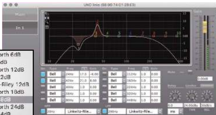
▲ Only two of the ten freely programmable EQ bands were needed to correct the bass for our listening room. The pull-down shows the high- and low-pass filters available.
