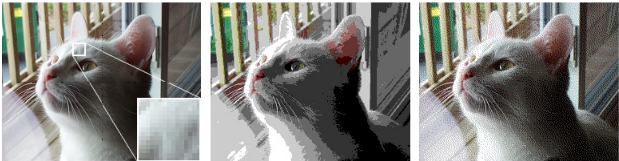
Figure 26: Image processing: original (left), quantized without dithering (middle), quantized with dithering (right)
