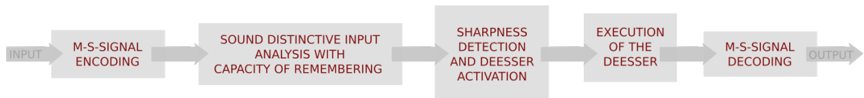
Figure 30: Block diagramm of the Weiss De-Esser plugin
